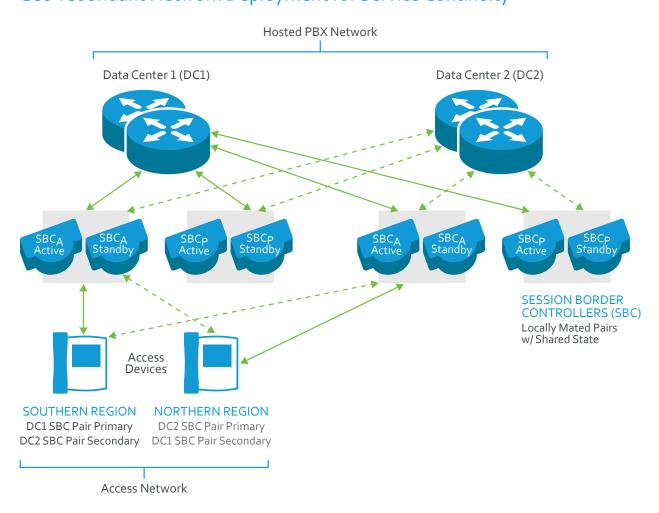
In the rare event a hosting data center is the point of failure, service will failover to the closest hosting data center and continue delivery with minimal impact to the organization leveraging the UC system.
